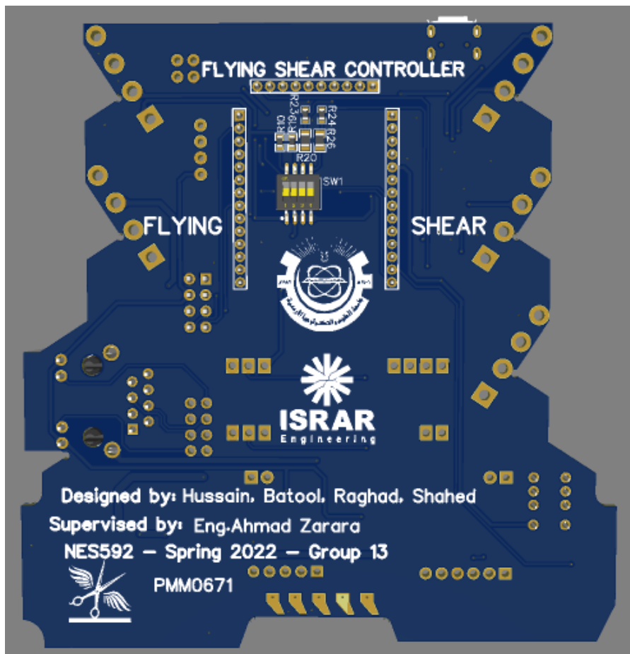
Figure 3.24. Bottom View of the PCB of Flying Shear Controller
